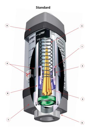
The flow meter is a variable area instrument. A sharp-edged orifice, located within the piston assembly, forms an annular opening with the contoured metering cone. The piston assembly carries a cylindrical PPS/ceramic magnet that is magnetically coupled to an external indicating magnet which moves precisely in direct response to movement of the piston. A calibrated spring opposes flow in the forward direction.
